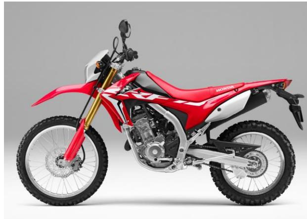
The 249cc engine boasts more bottom-end torque and peak power from revised PGM-FI and throttle body plus a new airbox, connector tube and lightweight exhaust.
